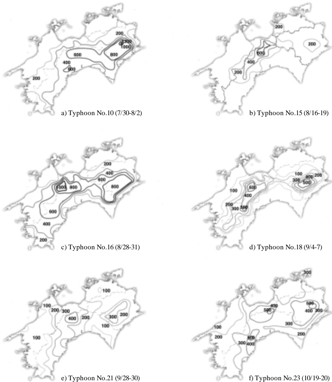
Figure 3 Iso-precipitation curves of Typhoons that attacked Shikoku Island in 2004 (rainfalls are the cumulated values of the days indicated in parenthesis) (* Documents proposed by the Japan Weather Association(JWA))
