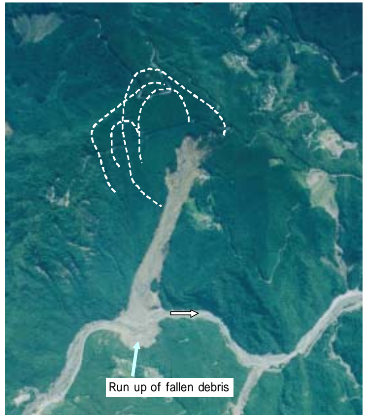
Photo 4 Aerial photograph of Azue area just after the occurrence of slope failure.
